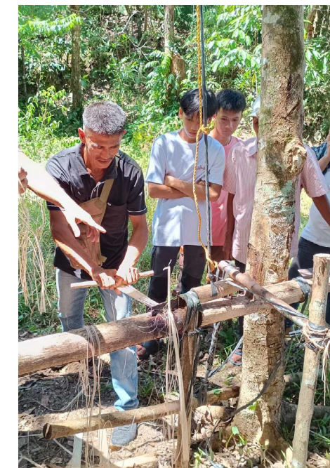
▲ The participants have a firsthand experience in separating banana pseudo stem using manual stripper.
