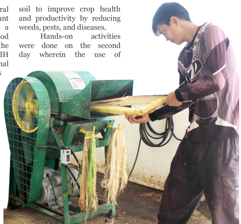
The demonstration of the process of fiber extraction from banana pseudo stem using decortivating machine.
